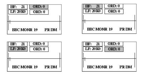
Use **UP/DOWN/LEFT/RIGHT** to select between Freq, Order relative to HP and LP (Butter worth). Dial changes selected values, while updating the graphics, the asterisk will be shown as above. The filter will be inserted into the signal path in real time (no confirmation needed).
